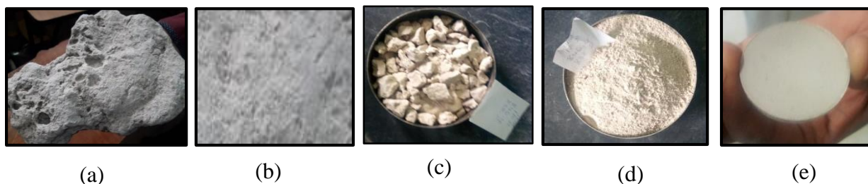
Figure 1: Sample preparation steps: (a) Matisaa gray rock deposit, (b) Cleaned portion of the rock, (c) Rock broken into grindable size, (d) Rock ground into powder and (e) Powder pressed into a pellet (diameter =22mm).
